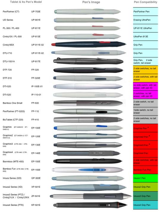
Usually the pens and other accessories are specific to the tablet model they come with. But there are exceptions. For the pens marked with the same color on "Pen Compatibility" column in this web page, they are interchangeable. Pens marked with different colors are not interchangeable.
